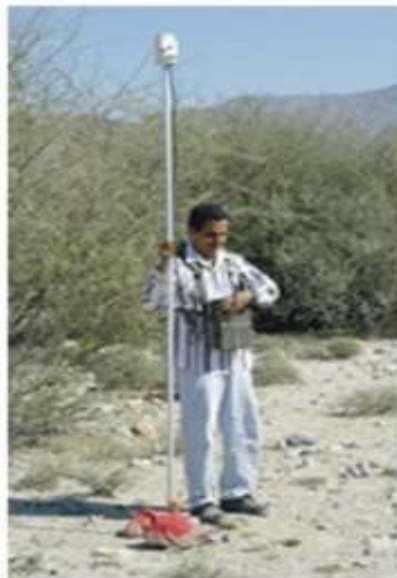
Figure 5: Magnetic measurement with proton magnetometer (Saudi Geological Survey)
