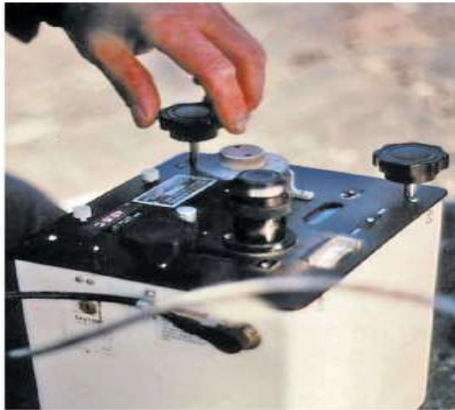
Figure 5: Land gravimeter (After Henry, 2010)
